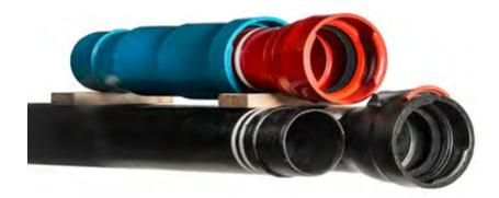
For Seismic Events including Liquefaction, Subsidence and Permanent Ground Deformation zones, the McWane Ductile SEISMIC FLEX COUPLING $^{\text{TM}}$  (SFC) provides state of the art resilience by significantly increasing joint deflection & axial expansion/contraction ranges above industry averages. The SFC will be utilized with the TR-Flex $^{\otimes}$  restraint joint to provide ERDIP resilience.
