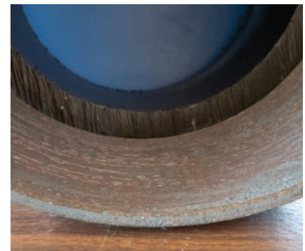
DI pipe (foreground) vs. HDPE (background) internal diameter.
