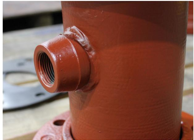
McWane Ductile utilizes Thread-O-Lets to allow for a broader range of threaded connections. These threaded connections are used where a direct tap is greater than the allowable size for a direct tap or not allowed. The pressure rating of the Thread-O-Let will be the same as the main/or adjoining pipe. The chart below shows the available Thread-O-Lets and their overall dimensions.
