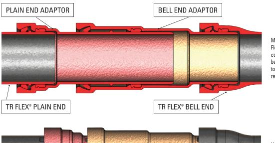
McWane Ductile's Seismic Flex Coupling™ is fully compatible with any TR Flex<sup>®</sup> bell or plain end, allowing it to be easily inserted into a restrained joint pipeline.
