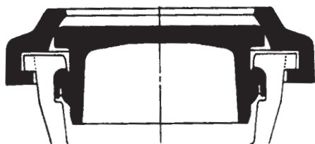
Section Showing Plug Installed in Bell
