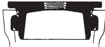
Push-on Plug Installed
