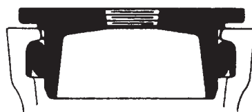
Push-on Plug Installed
