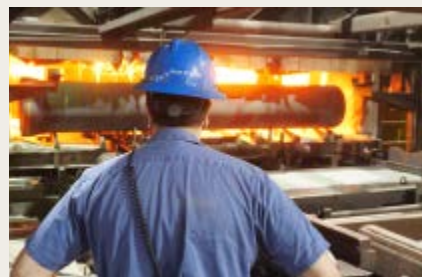
Ryan Rinkes — MDO Finishing Supervisor, monitors the annealing oven.
