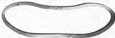
Ring section cut from 12-inch ductile pipe, which has been squeezed under hydraulic pressure to show how metal bends without breaking.
