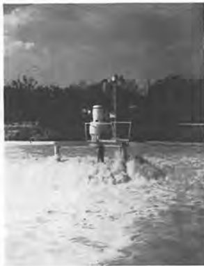
Tough paper waste aerated with float-mounted Sigma
