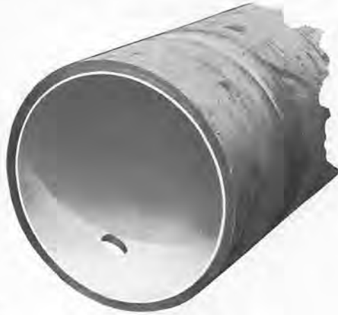
Photograph of a cement lined cast iron pipe (without seal coating) that has been cut and tapped, showing how the cement lining does not spall off in either operation.
