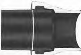
Cutaway of the joint completely assembled, showing the stripe no longer visible.
